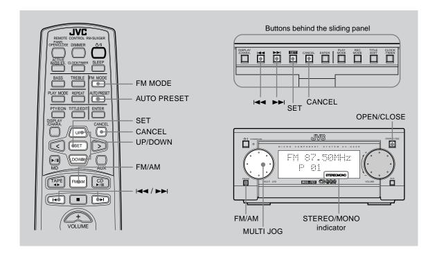
You can tune in FM and AM (MW/LW) stations manually, automatically, and use the preset station feature.
